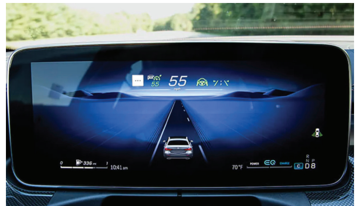
With the active driving assistance system engaged in the 2022 Mercedes-Benz C-Class, the driver’s instrument panel shows the car within the lane lines, while the green steering wheel with hands icon indicates that lane centering assistance is functioning. Photo: John Powers/Consumer Reports
